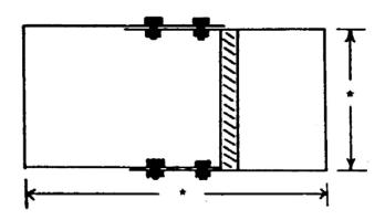
Sampler is placed in the uncompacted lift directly behind paver and all material is removed.
